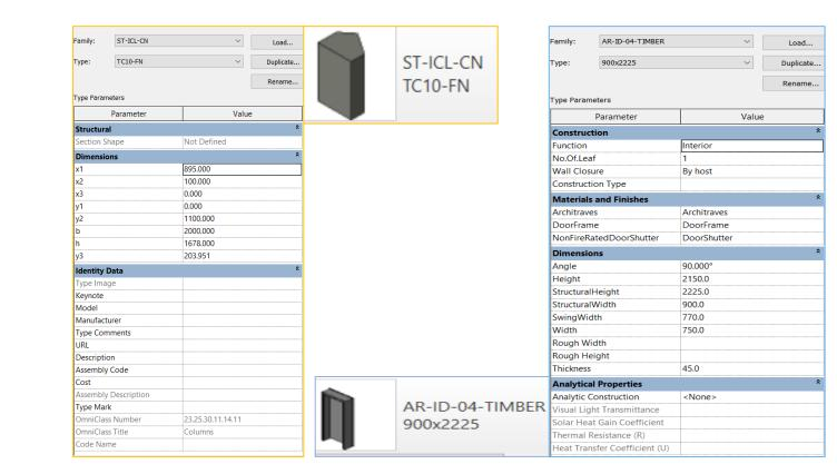
Construction Operations Building Information Exchange (COBie) is a non-proprietary data format for the publication of a subset of building information models (BIM) focused on delivering asset data as distinct from geometric information
