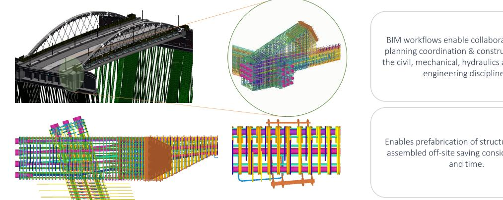
BIM workflows enable collaborative design, planning coordination & construction across the civil, mechanical, hydraulics and electrical engineering disciplines.
