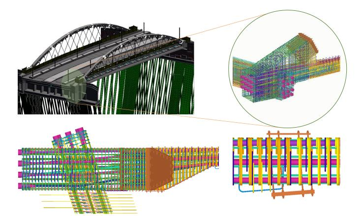
BIM workflows enable collaborative design, planning coordination & construction across the civil, mechanical, hydraulics and electrical engineering disciplines.
