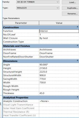
Construction Operations Building Information Exchange (COBie) is a non-proprietary data format for the publication of a subset of building information models (BIM) focused on delivering asset data as distinct from geometric information
